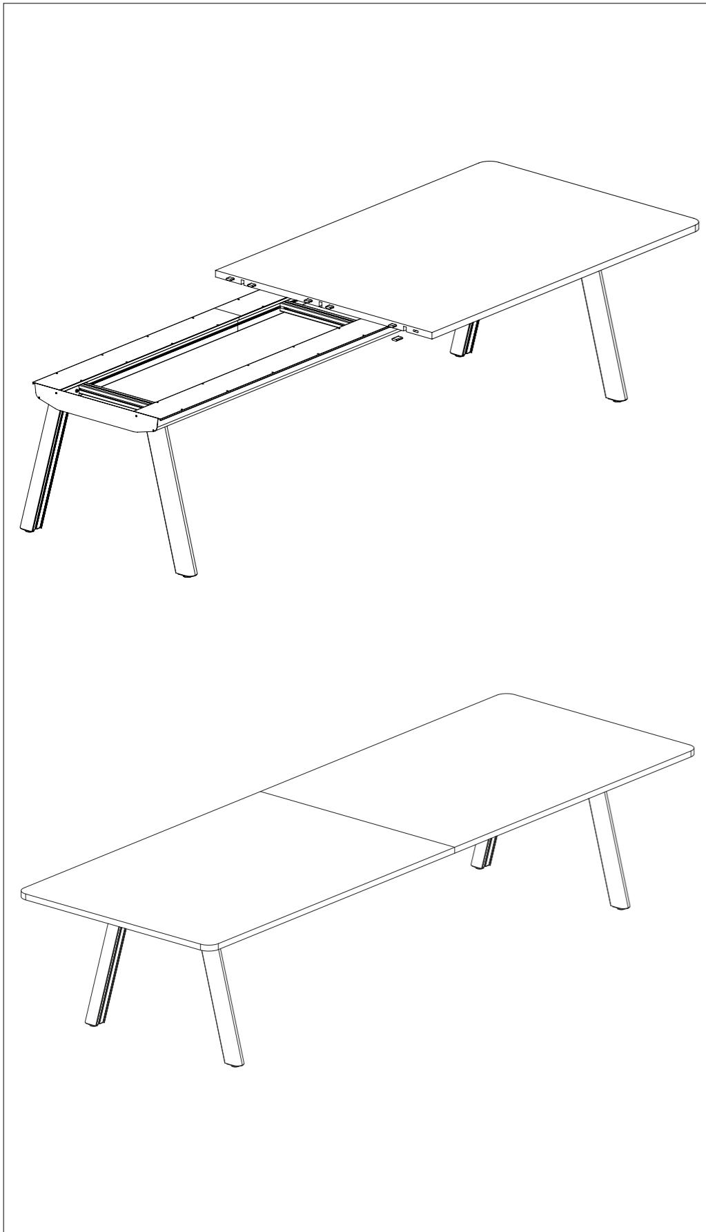
11 Insert tabletop connectors underneath the tabletop
