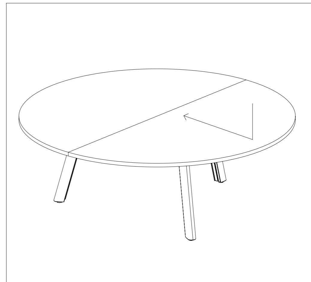
Place the second tabletop part onto the frame, align it and push the two sides together so the tabletops are leveled.
