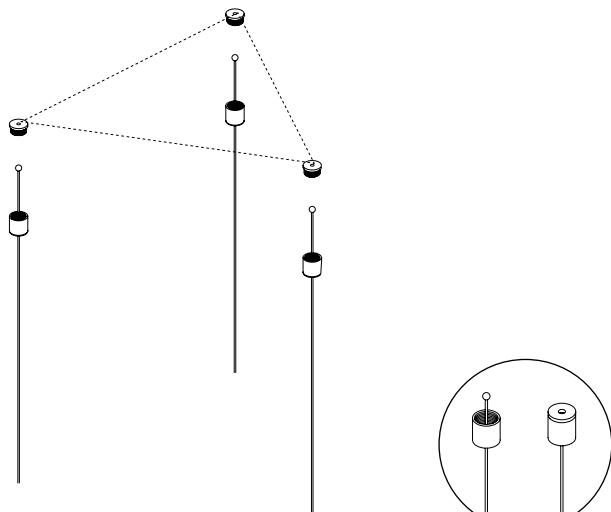
5 Push the three steel cables into the cable adjusters and adjust them to the desired height. Make sure to thread the steel cable through the transparent o-rings on the electrical cord
