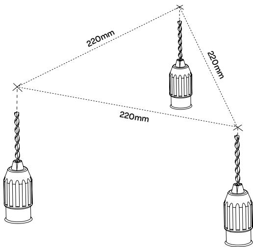
3 Insert plugs and screw the ceiling disk onto the plug.
