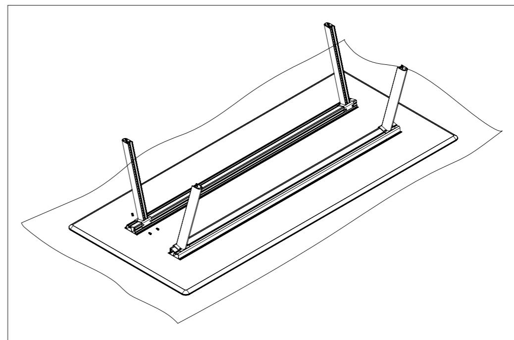
Connect the table legs to the profiles with 4x M8x16 bolts per leg using the allen key
