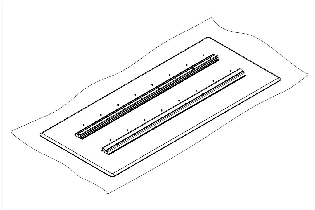
Place profiles on the backside of the tabletop and mount them using PZ 5x16 screws.
