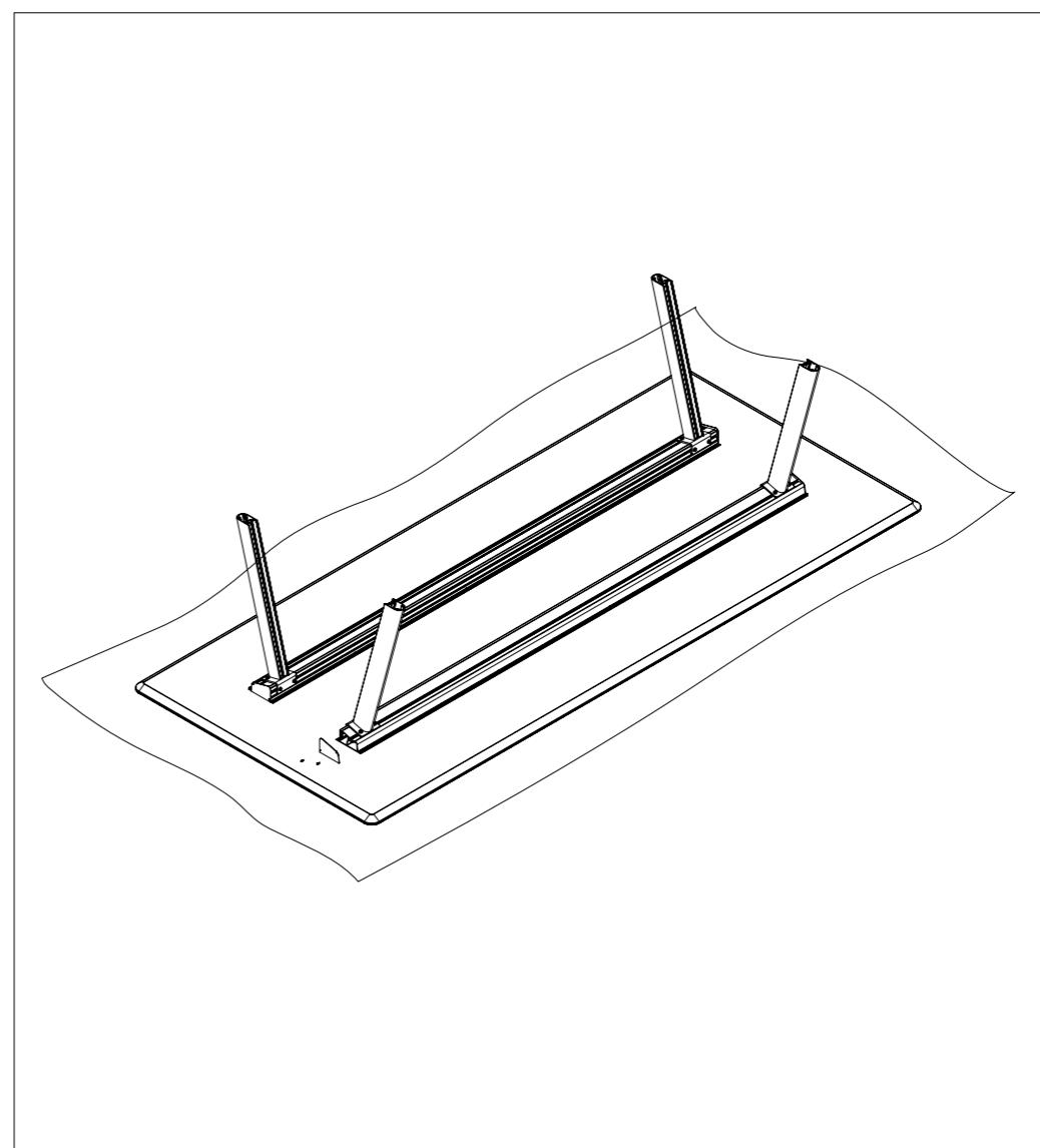
Place 1x frame cover per head side of the profile and fasten it with 8x self-tapping screws M3x10
