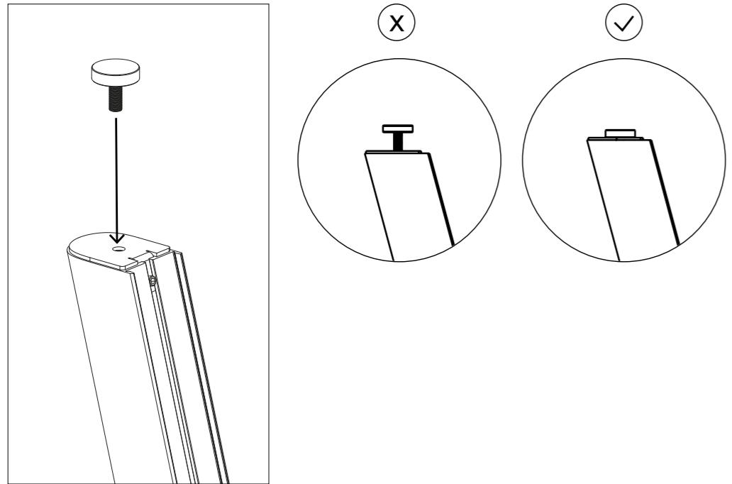
Please, take into account that adjustable feet are intended for levelling the tabletop and not for height adjustment.
