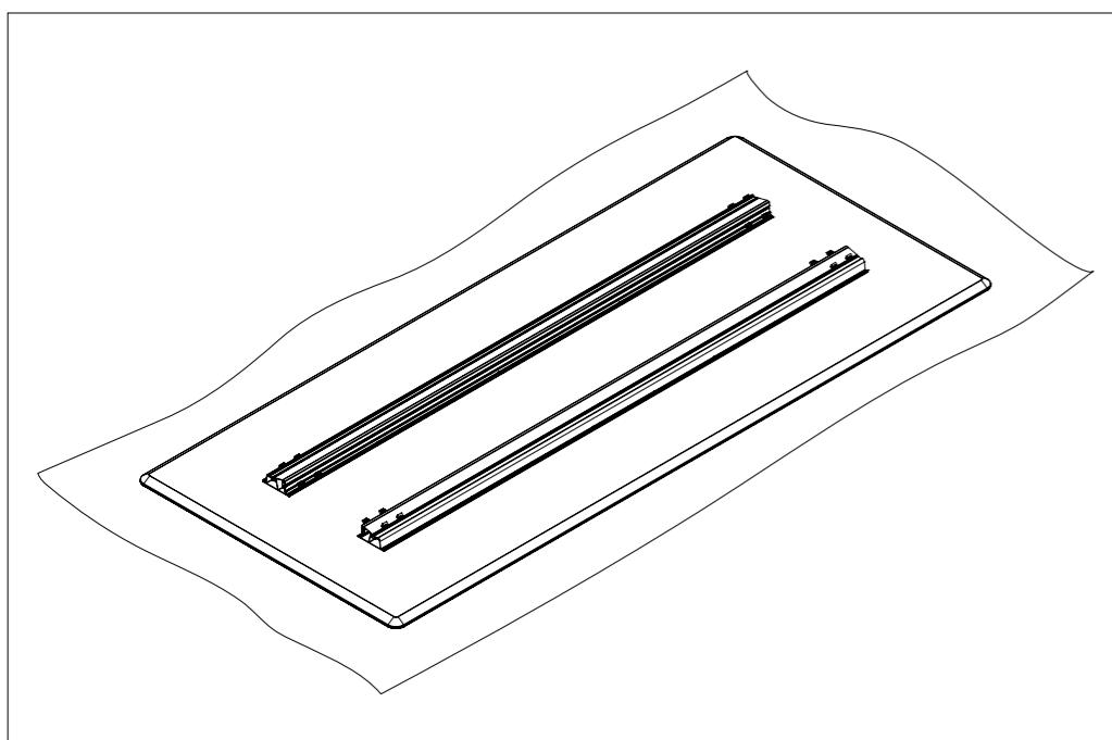
Insert 4x M8 sliding nuts at each end of the profiles
