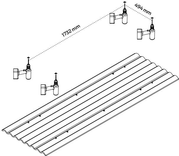
5 Install the ceiling cap and connect the steel wires to the holes in the ceiling.
