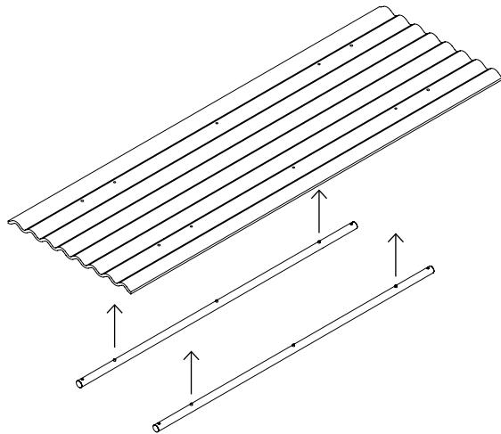
2 Mount lighttubes on the panel with the screws together with the Countersunk washer.
