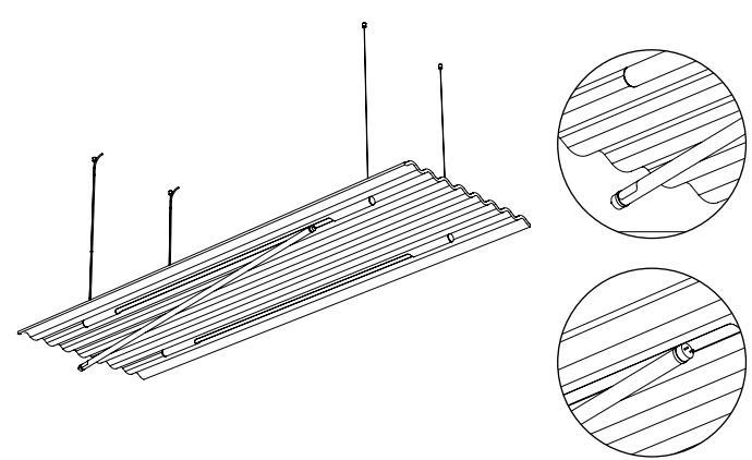
7 Slide the light diagonally into the LED tube.
