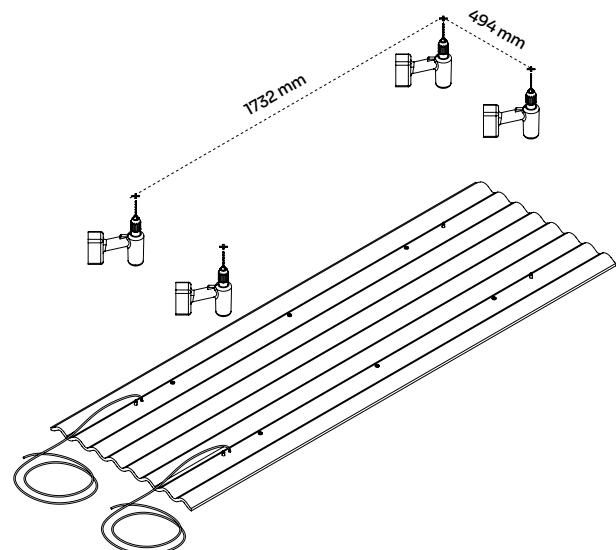
5 Install the ceiling cap and connect the steel wires to the holes in the ceiling.
