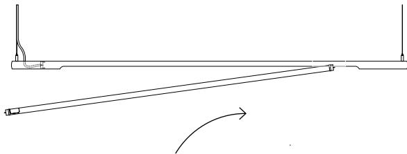
8 Slide the light horizontally as far as possible into the tube.
