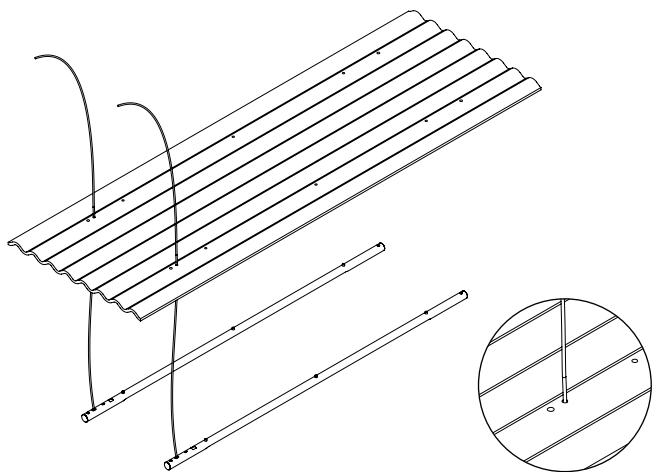
2 Mount lighttubes on the panel with the screws.
