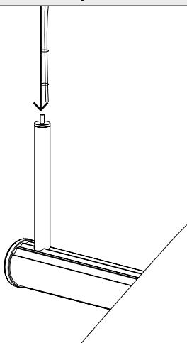
6 Adjust the steel cables accordingly by pushing the cable gripper down to lower the lamp.
