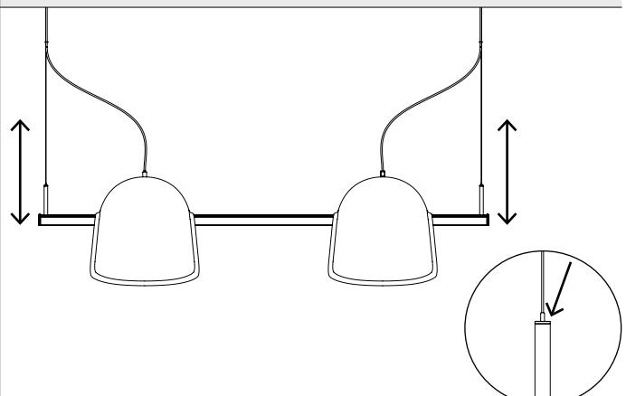
7 Connect the lamp to the power supply and you are all set! To adjust the direction of light, hold the horizontal rail while turning the lampshade into desired position. The lampshade can be set into 5 positions.
