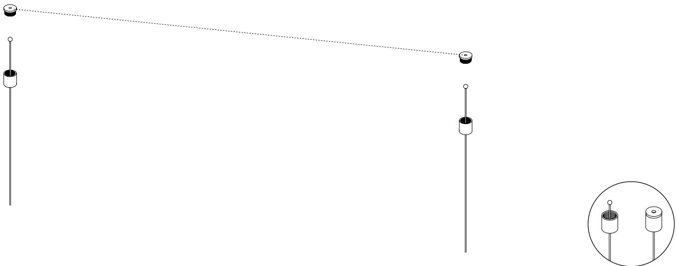
5 Cut the steel cable to the desired length. Thread the steel cable through the rubber rings on the cord and push the steel cables into the cable adjusters.
