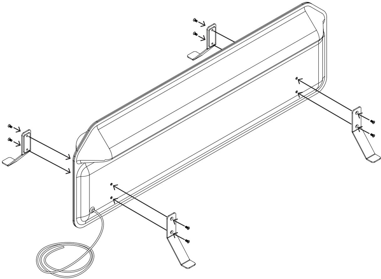
4 Tighten the screws on both sides. Use two identical allen keys.
