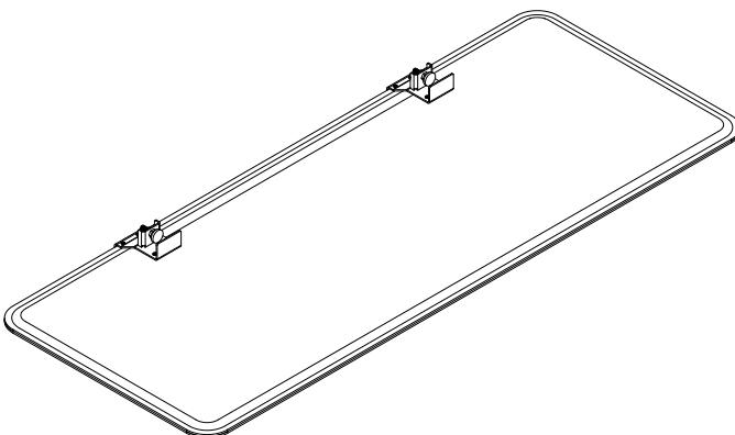
7 Mount the panel onto the tabletop and fix it using the adjustable feet (you can use a wrench or a hex key).
