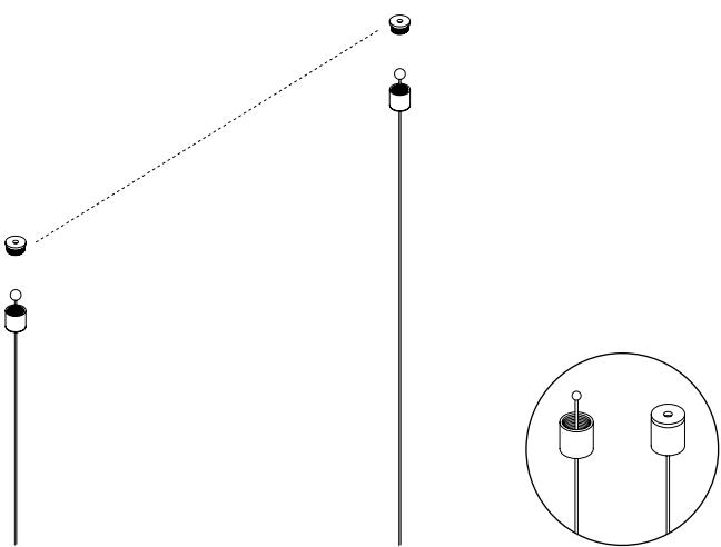
5 Push the 2 steel cables into the able adjusters and cut off the excess cable.
