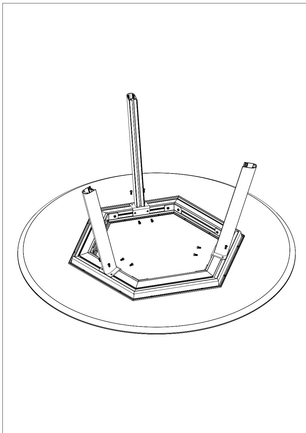
Connect the table legs to the profiles with 4x M8x16 bolts per leg using the allen key.
