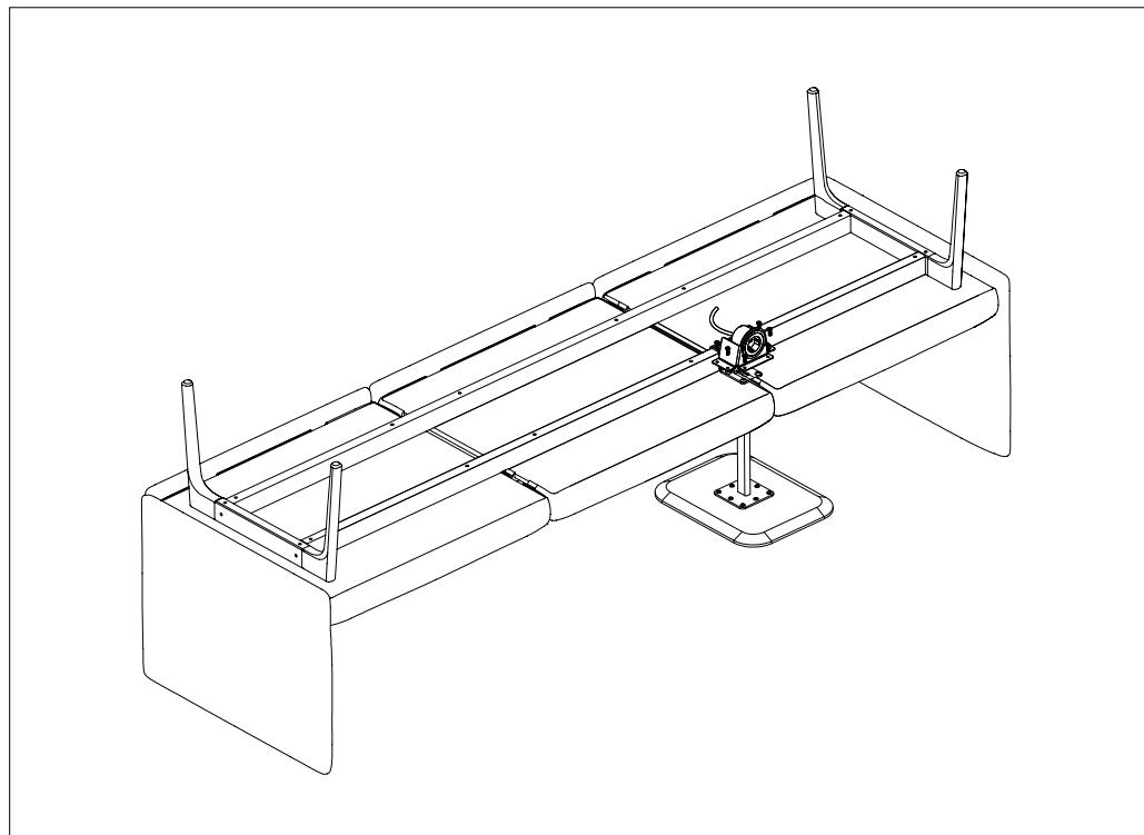
Place the electrification bracket at the desired position. Use a power drill with magnetic bit holder to attach the bracket to the frame using (6x) buttonhead screws PZ 5 x16.
