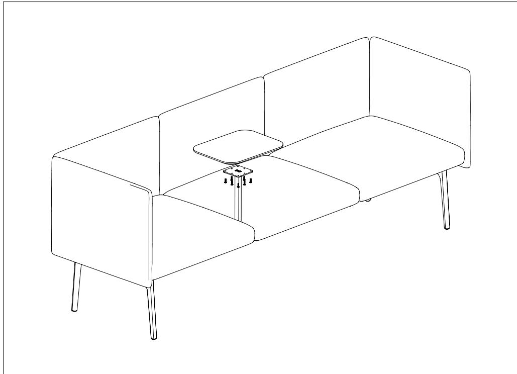
Place the tabletop on the base and attach it using (8x) button head screws PZ 5 x 16. Use a power drill with magnetic bit holder to mount the screws.
