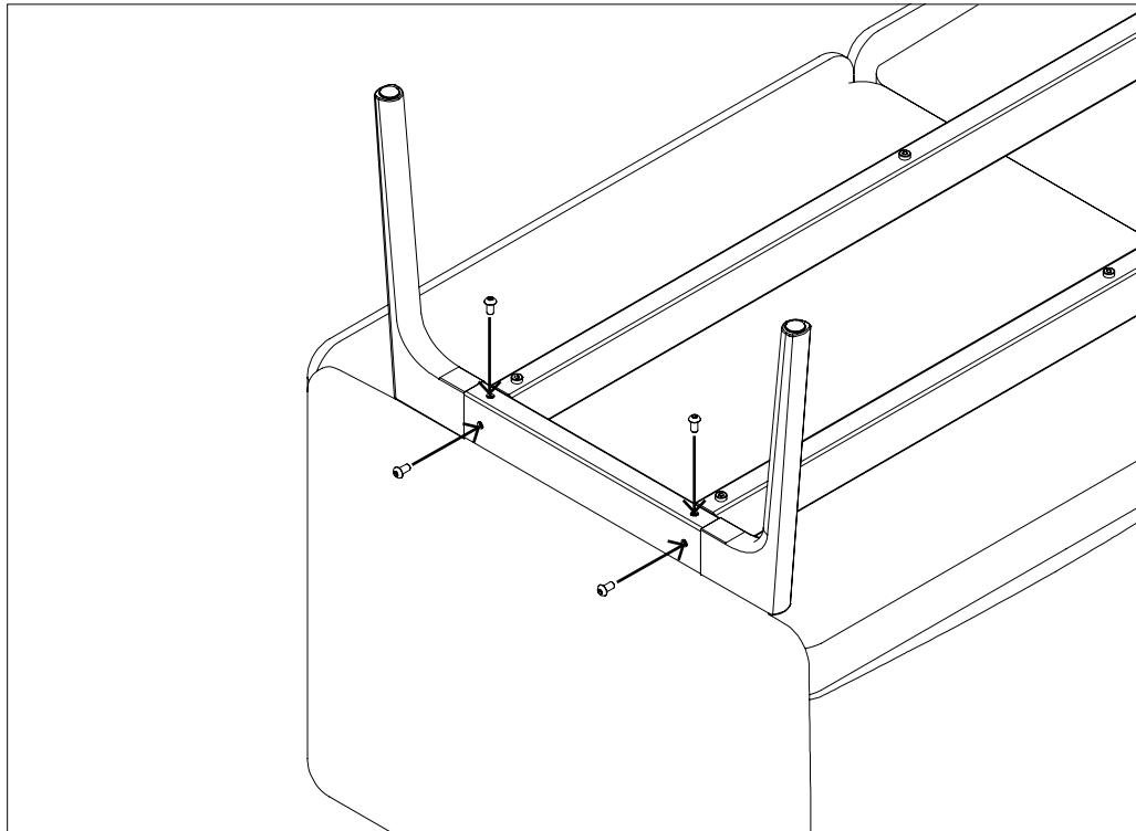
Use an allen key to mount the (2x) screws M6 x 12 mm per leg.
