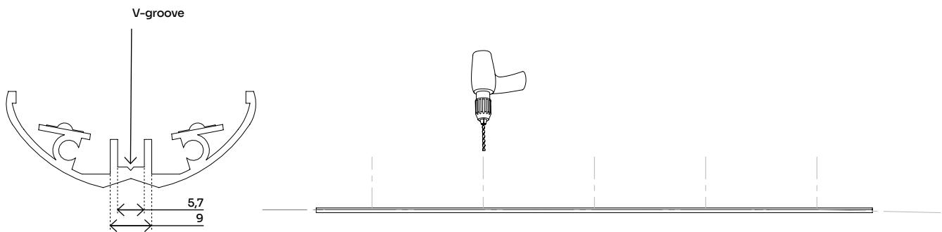
**4** Secure the LED profile to the wall with the top screw. Use a spirit level to position the LED profile so its perfectly level.
