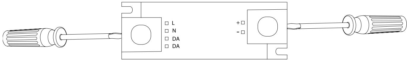
8 Connect the LED cables by pushing a small flathead screwdriver into the push-in terminals.
