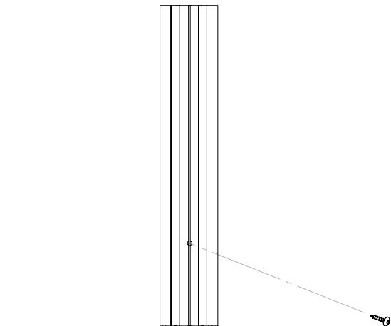
**4** Once the profile is level, fasten the remaining screws.
