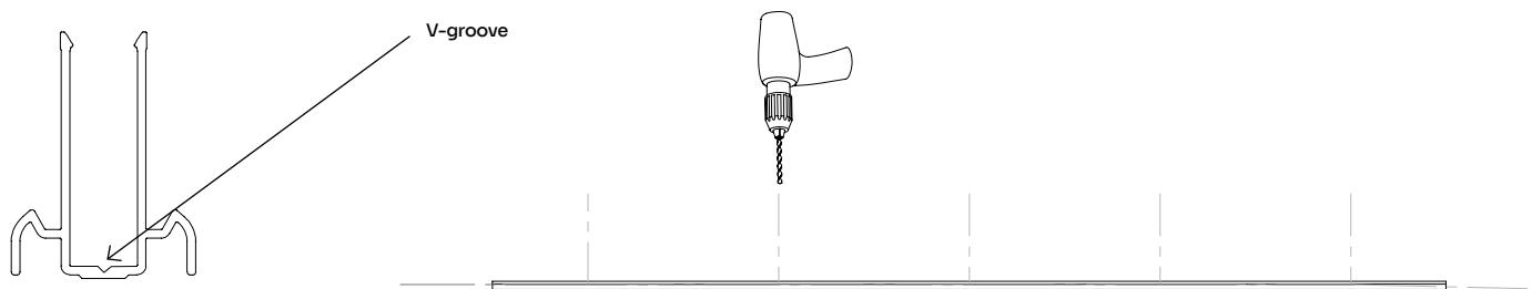
**3** Secure the wall profile to the wall with the top screw. Use a spirit level to position the wall profile so it is perfectly level.
