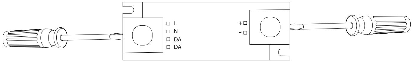
9 Connect the LED cables by pushing a small flathead screwdriver into the push-in terminals.
