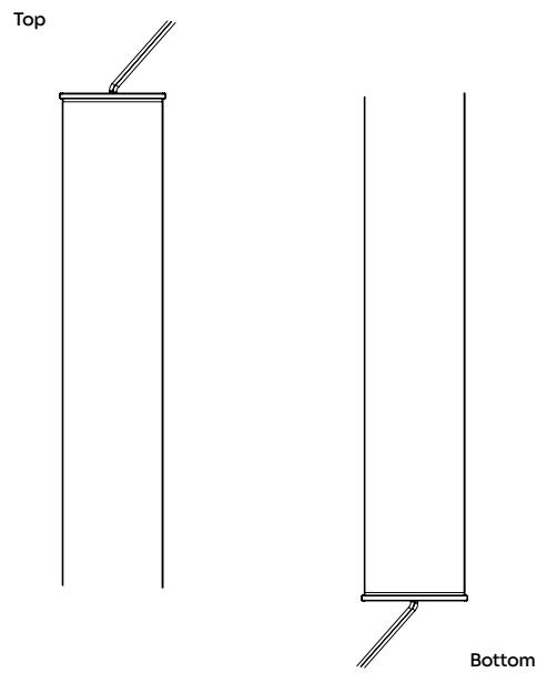
6 - Place the LED profile on one side inside the wall profile
