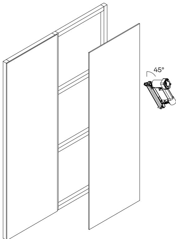
Test the pressure of the nail gun and adjust it, so that the nails don't go too deep into the material.
