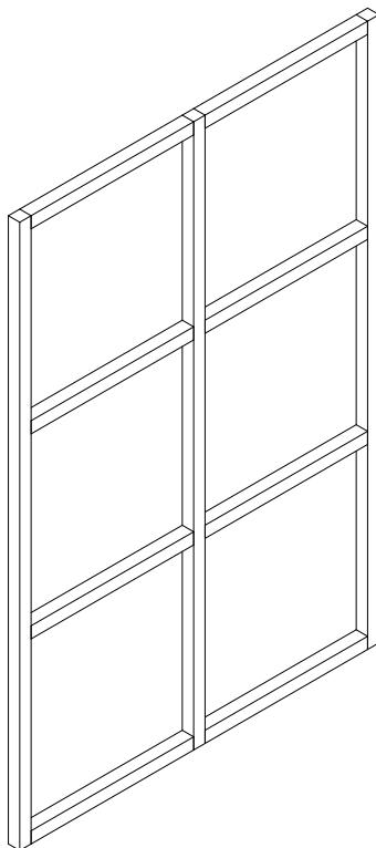
A wooden framework is necessary if you install the panels using a nail gun.
