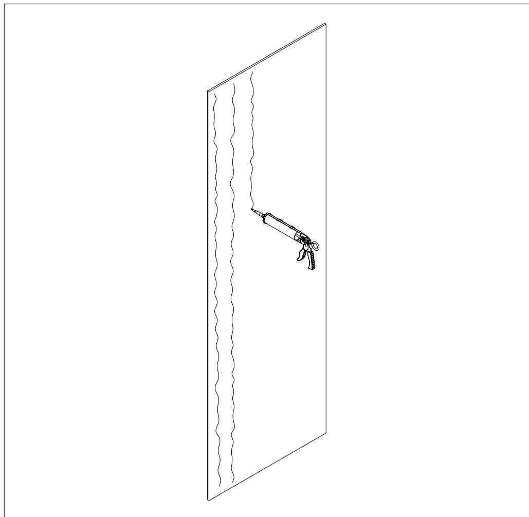
Apply the adhesive on the backside of the panel following the manufacturer's instructions.
