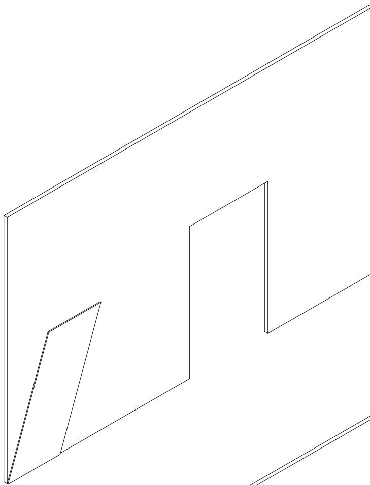
Place the panel against the surface, starting at the bottom. Make sure it is properly aligned using a level.
